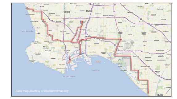
12" - 36" Pipelines (Crude Oils and Vacuum Gas Oils)
